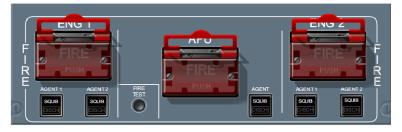
4 Press engine(s) and/or APU AGENT pushbuton(s) as required
